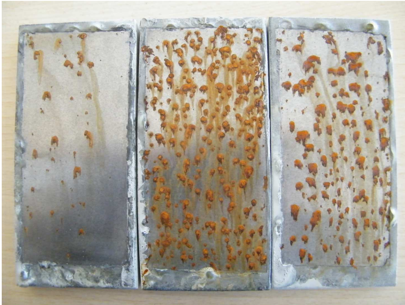
Salt fog testing of wire sprayed steel coatings
